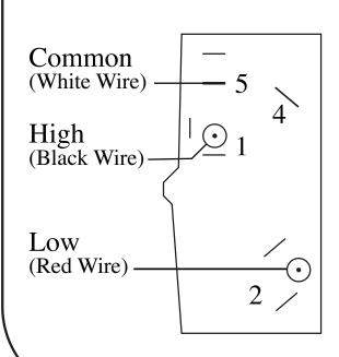
White Wire – to be connected to common terminal on motor
